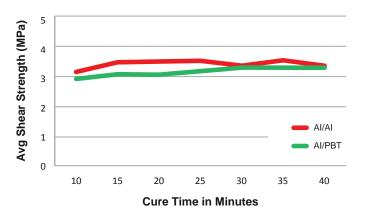
Lap shear, 7-mil (178um) bondline, Ticona® 3300D PBT (30% GF), 2"/minute (0.8 mm/s) rate on Tensometer.
