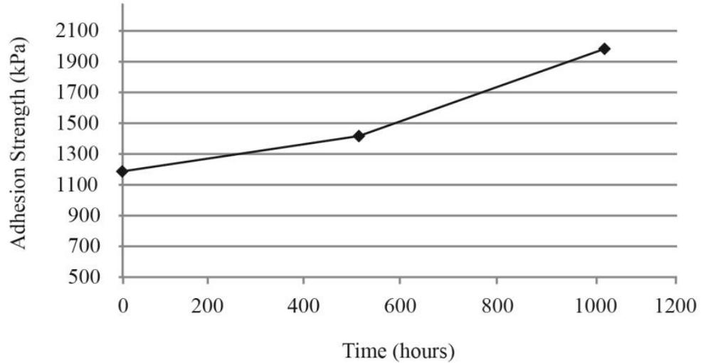
DOWSIL SE 1720 CV Adhesive Adhesion Strength Over Time during 150°C Exposure
