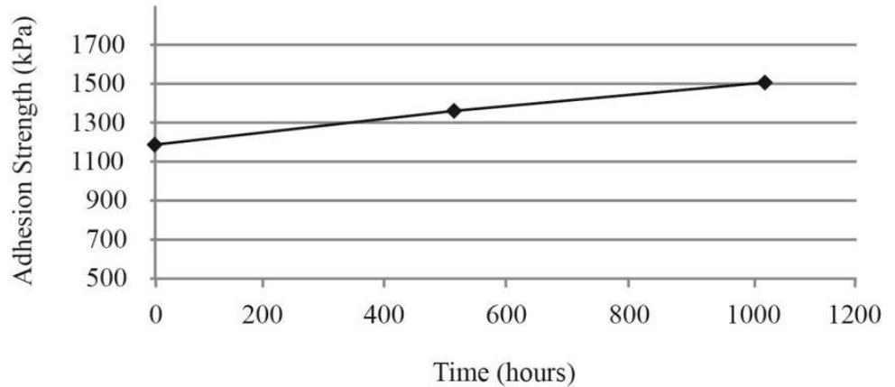
DOWSIL SE 1720 CV Adhesive Adhesion Strength Over Time during 85°C/85% RH Exposure
