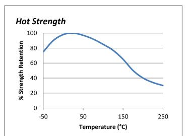
"Hot strength" shear strength tests performed on mild steel. Initially cured at room temperature and then post-cured at 150°C for 2 hours. Test pieces conditioned to pull temperature for 30 minutes before testing.
