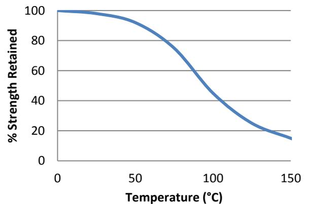
"Hot strength" shear strength tests performed on glass to mild steel. Fully cured specimens conditioned to pull temperature for 30 minutes before testing at temperature.
