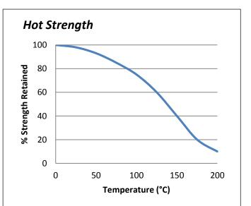
"Hot strength" shear strength tests performed on glass to mild steel. Fully cured specimens conditioned to pull temperature for 30 minutes before testing at temperature.
