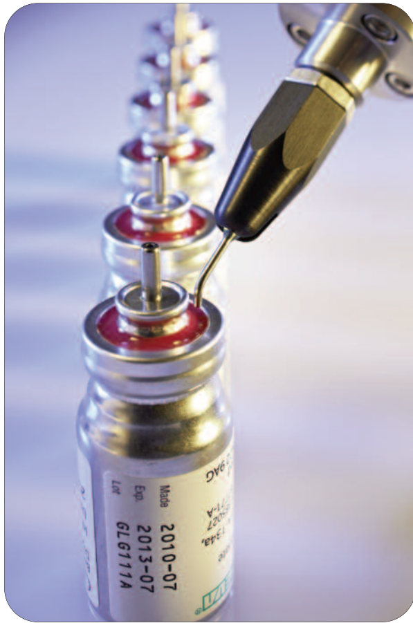
TS5440 - dispensing medical device adhesive
