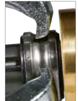
Lock on ball grooves and bearing races.
