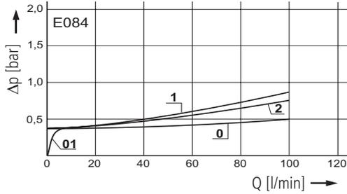
Pressure drop as a function of the **kinematic viscosity**
