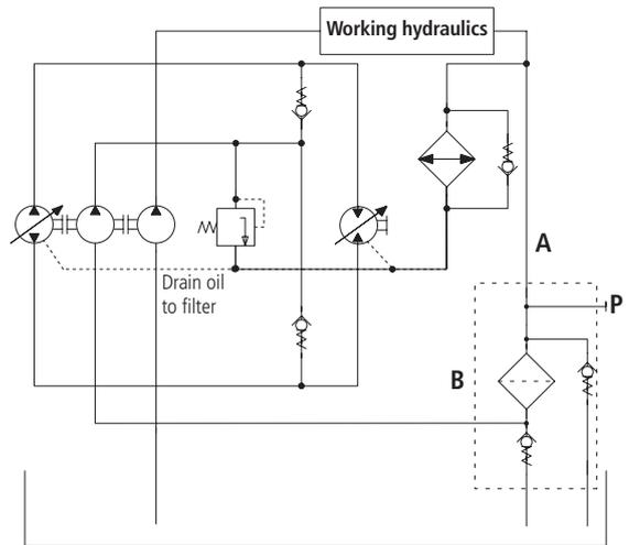
The entire dirt produced in the hydrostatic drive by abrasion is filtered out immediately and is thus not taken in by the pump of the open-loop circuit.
