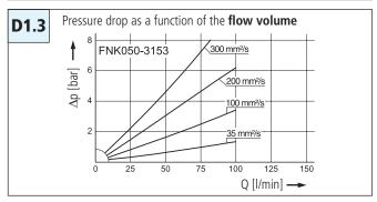
In general the pressure drop increases in line with a larger cooler length. Exception:
