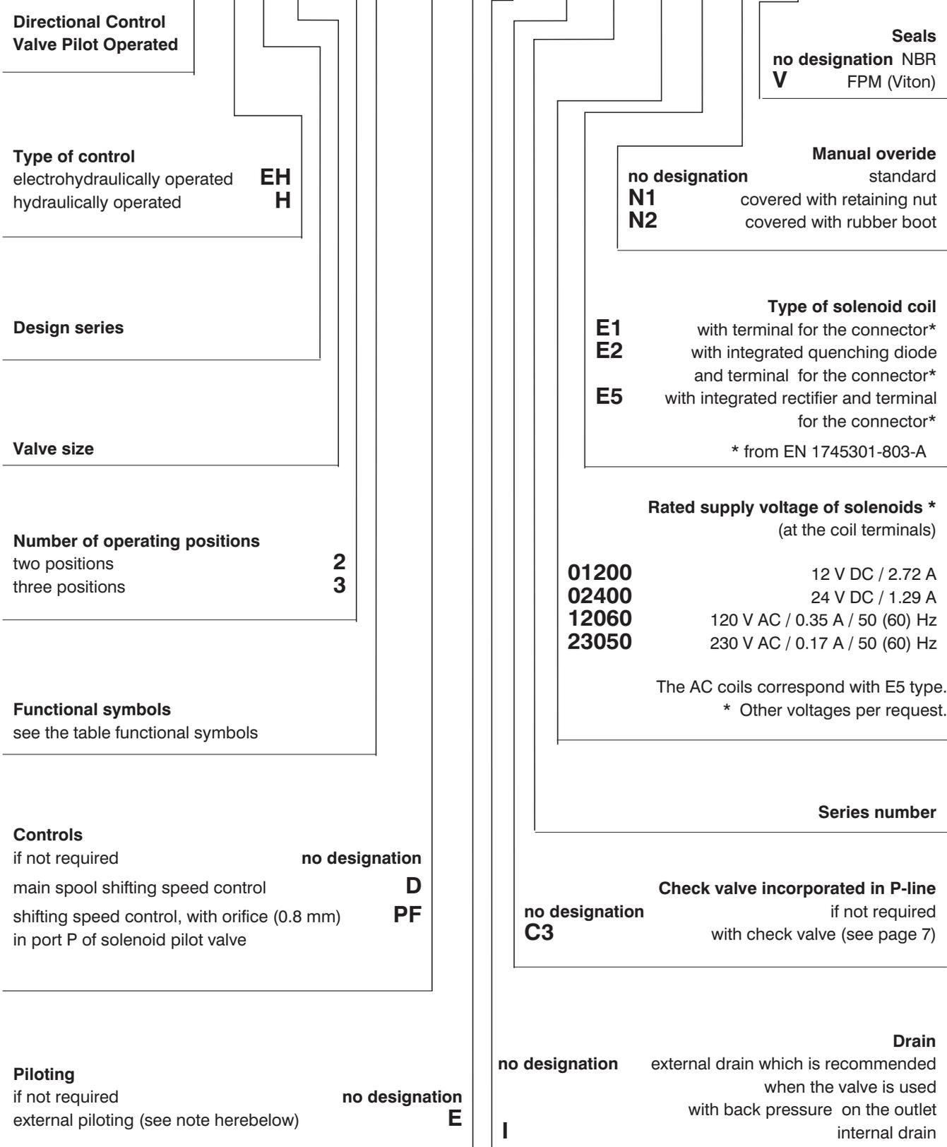
**Directional Control Valve Pilot Operated**
