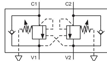
The use of aluminium bodies is limited to a maximum operating pressure of 210 bar.
