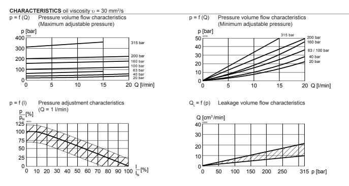
Adjustable range of nomial pressure, adjusted with set screw under the clamp cap.
