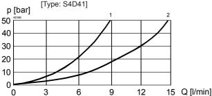
Q = f (s, x) Volume flow-signal-characteristics ( $\Delta p$  = 10 bar) [Type: S4D41]
