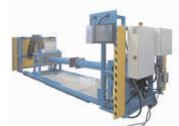
Central Coupler Testing Machine
