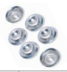
1/4" angular seat rupture discs are designed to be used with the safety head assemblies that are shown above. Minimum rupture disc pressure ratings should be at least 110% of system operating pressure. The standard material is stainless steel. The pressure ranges indicated in the table below are at room temperature (72°F). Other materials and pressure ranges are available upon request.
