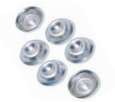
$^{1/4}$ " angular seat rupture discs are designed to be used with the safety head assemblies that are shown above. Minimum rupture disc pressure ratings should be at least 110% of system operating pressure. The standard material is stainless steel. The pressure ranges indicated in the table below are at room temperature (72°F).Other materials and pressure ranges are available upon request.
