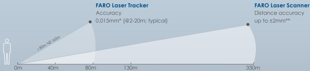
The **FARO Laser Tracker** is a portable 3D measurement system for large volume which uses laser technology and Absolute Distance Meter (ADM & IFM) to effectively and accurately measure large parts, tooling and machinery.
