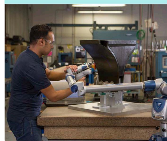
\*Repeatability = Single point articulation performance test. \*\*Accuracy = Volumetric maximum deviation. Performance specifications according to B89.4.22 (According to VDI/VDE 2617 Part 9 on request).
