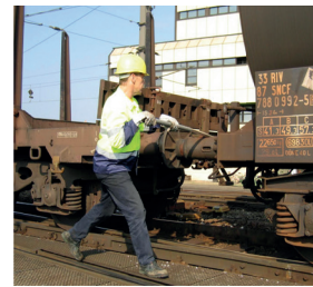
Fig. 2: shunter lifting the coupling
